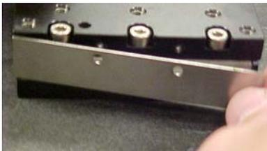
**Step 3:** Gently slide the bracket from out from under the carriage.
