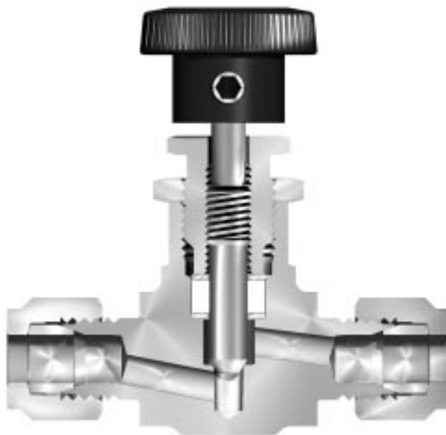
Figure 1: VL Series Needle Valve Cross Sectional View
