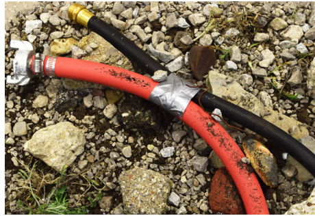
Tape hoses together
