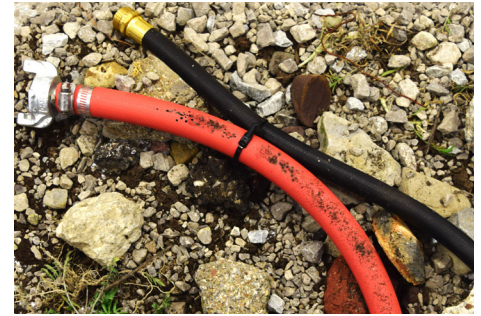
Zip tie or strap hoses together
