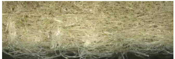
Cross section shows some dust penetration ~50% into the depth of the fabric.
