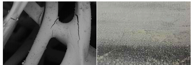
Fiber cracks, 1400x.
