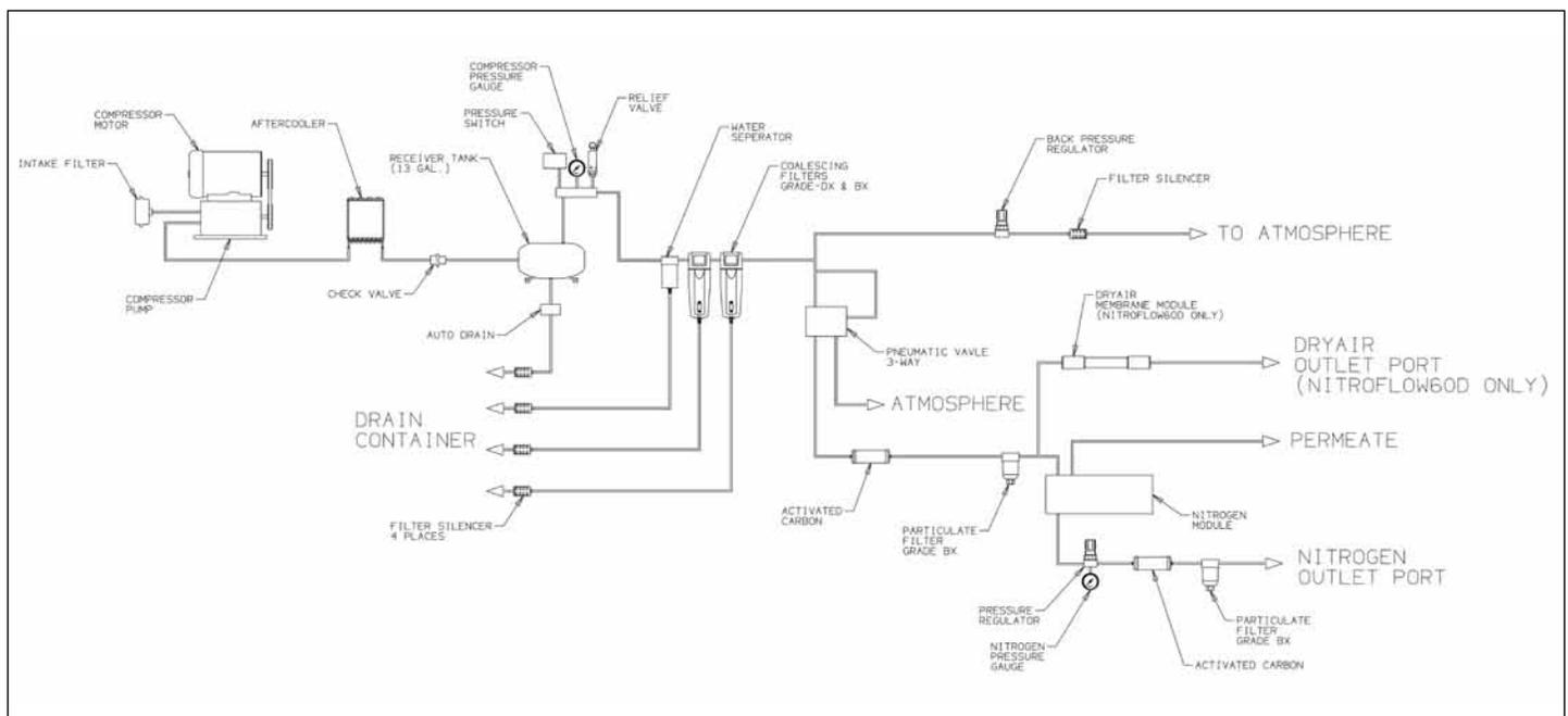
**Figure 1: Schematic Diagram of Nitroflow60 Nitrogen Generator**
