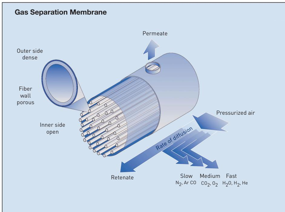
**Figure 2: Separation of nitrogen via a semi-permeable membrane.**
