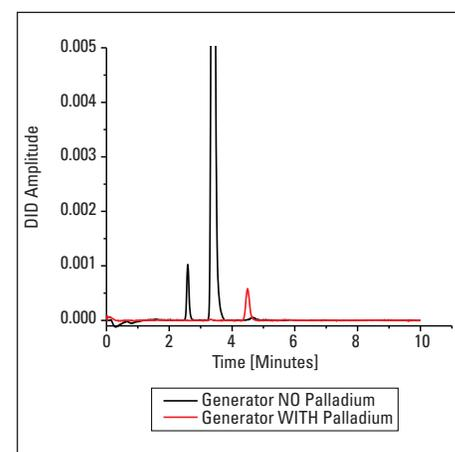
**FIGURE 4.** GC-FID chromatogram. Black line—generation of hydrogen with a system with palladium membrane as the final purifier. Red line—generation of hydrogen with a generator using a desiccant as the final purifier.
