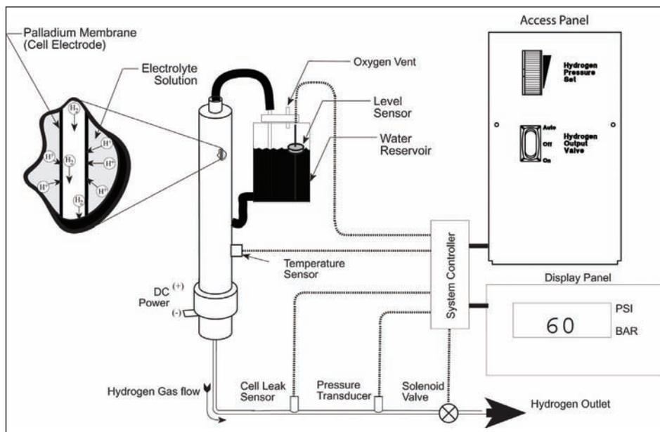
**FIGURE 3.** Overall design of a system for the generation of hydrogen via the electrolysis of water using a metal catalyst. Photo: Parker Hannifin Corp., Haverhill, MA
