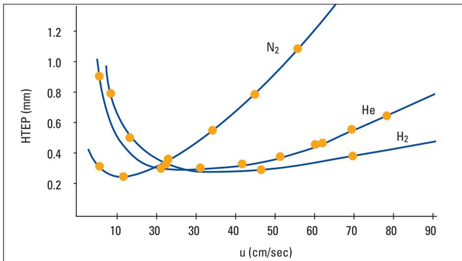
**FIGURE 1.** Van Deemter Plot for  $N_2$ , He and  $H_2$ . While  $N_2$  provides the highest chromatographic efficiency, the optimum velocity for  $H_2$  is considerably greater, so the use of  $H_2$  as the carrier gas can lead to analysis times that are four times faster than when  $N_2$  is used.
