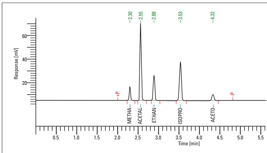
**FIGURE 5.** Headspace GC analysis: HS conditions - Oven 60 C, needle 65 C, pressurization time 3 min, injection time 0.04 min, 110 C transfer line temperature. Purge and carrier gases are hydrogen. GC: 40 C for 5 min, 25 C/min to 100 C hold 1 min; 25 C/min to 200 C. Column flow is 1.50 mL/min and injector is 200 C. Compounds are methanol, acetaldehyde, ethanol, isopropanol, and acetone. Photo: Restek, Inc.
