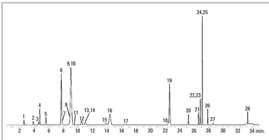
**FIGURE 2.** Headspace GC separation of 28 Class 1 and Class 2 residual solvents for pharmaceutical processing. Gas =  $H_2$ . Samples shaken and heated at 80 C for 15 min; 1 mL used for headspace injection. Photo: Restek, Inc.
