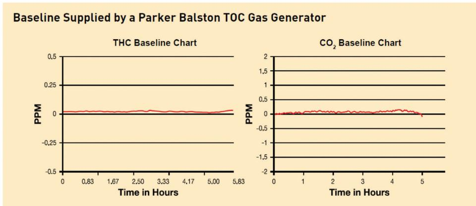
◀ *Figure 4. Baselines observed on a TOC analyzer from carrier gas from a Parker Balston generator. Left: total hydrocarbons; right: CO<sub>2</sub>*
