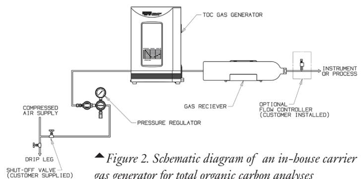
▲ Figure 2. Schematic diagram of an in-house carrier gas generator for total organic carbon analyses
