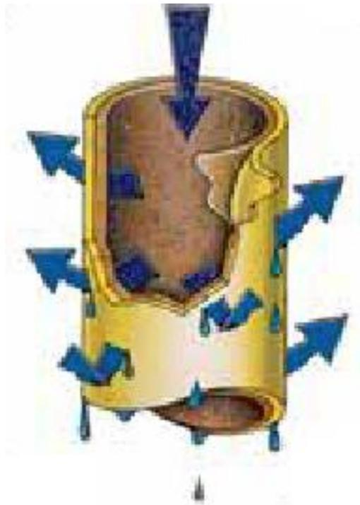
Figure 2 Permeation Membrane – Used to remove water vapor from air. The membrane bundle contains a large number of membranes to provide enhanced
