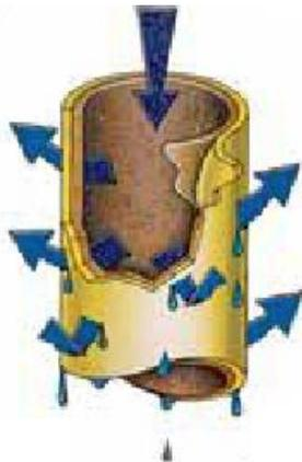
**Coalescing Filter** – Used to remove oil and water droplets, particulate matter from compressed air. The liquids drip to the bottom of the filter housing and are automatically emptied by a drain assembly.
