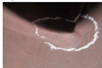
**30. LP baffle** reveals protective oxide coating and no signs of FAC or oxygen pitting
