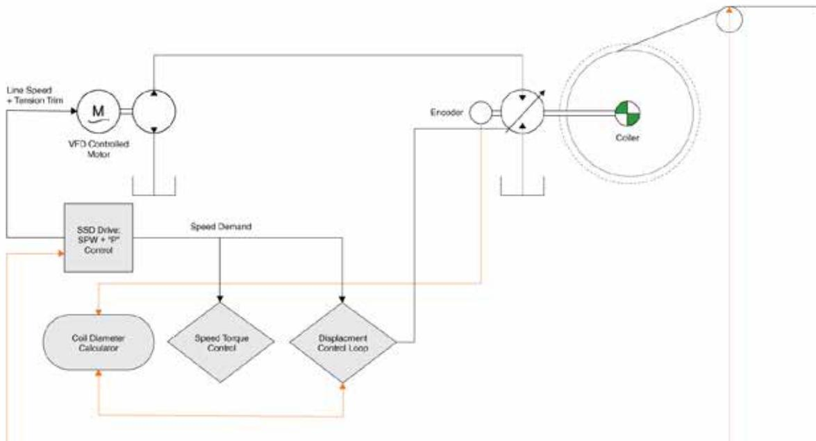
Diagram 1: Simplified DCP Coiled Circuit
