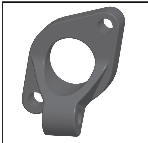
The composite bracket is a direct replacement for the zinc alloy version and will fit all existing sections in the field. This bracket uses the same two cap screws, but the torque value has been changed to 4-6 ft lbs. This is the same torque as used on the composite bonnet (torque value for the zinc and cast bracket is 10 ft lbs).
