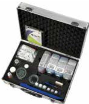
**The DIGICell is the essential device for Water in Oil and BN (Base Number) testing - now tests up to BN150!**
