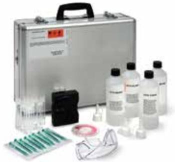
**The Cold Corrosion Test Kit (CCTK) provides an accurate measurement of corrosive iron content in cylinder liner oil.**
