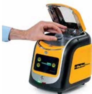
**The ability to spot check the Sulphur content of fuel on-board (to lab standards) within three minutes will help vessel operators, bunker suppliers, port authorities and regulatory surveyors ensure compliance with the latest IMO MARPOL fuel regulations.**
