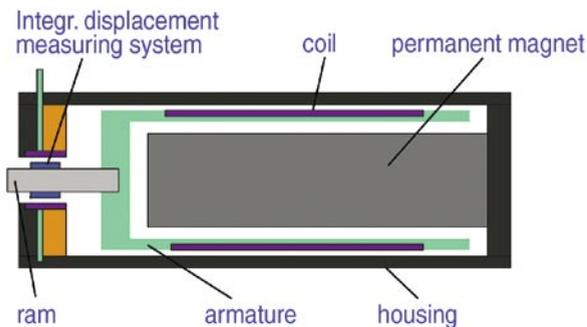
The directly coupled spool drive has a displacement measuring system at the transition. Together with the onboard electronics, highly dynamic and precise position controllers can be constructed.
