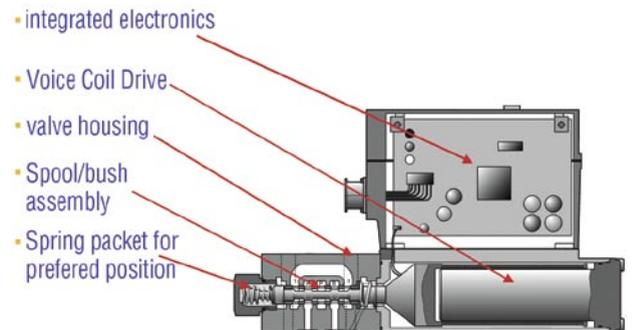
The Voice Coil Drive is based on a movable plunger coil, which surrounds the fixed magnet. When current is applied by means of the onboard electronics, this valve drive develops a force of up to 100 N.
