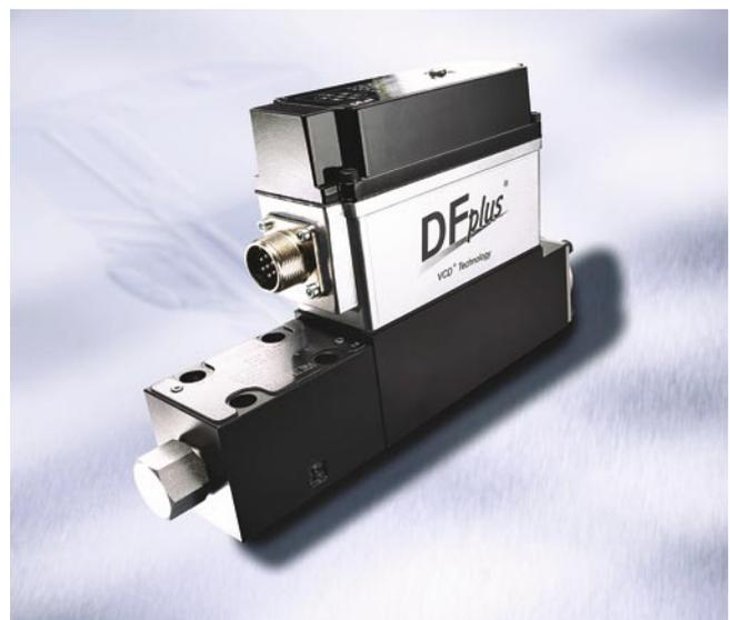
*The valve spool actuator, an innovation in the field of hydraulics, provides the DF<sup>plus</sup> with a response time of 3.5 ms. In this time, the spool covers 90 percent of its deflection.*
