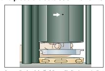
Lower the back half of the split die ring onto the dies by pulling the slide pin forward.
