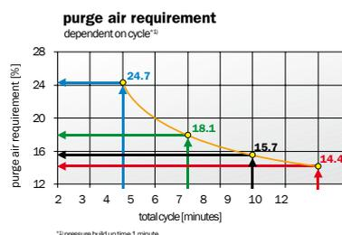
The Parker Zander 10-minute cycle with an adsorption time of 5 minutes leads to 12 load alternations per hour. The customary 6-minute cycle with an adsorption time of only 3 minutes requires 20 load alternations per hour. The consequence: Parker Zander dryers save 5.6 % of regeneration energy.
