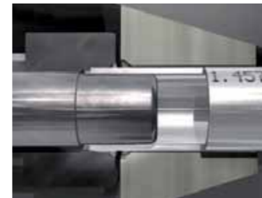
2. Tube is inserted into the tools until it firmly touches the stop at the end
