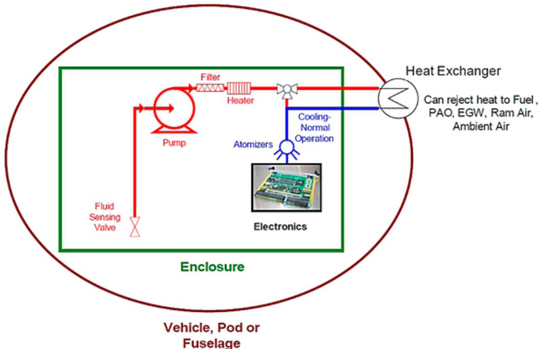
**FIGURE 1. SYSTEM DIAGRAM OF DIRECT SPRAY ENCLOSURE**
