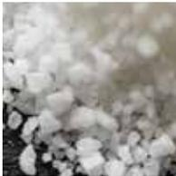
Sodium sulfate ( $\text{Na}_2\text{SO}_4$ ) is present in sea salt, but most often occurs when sodium chloride and sulfur react during combustion. The sulfur is almost always supplied by the fuel, while the sodium chloride can be the result of contaminated fuel or insufficient inlet air filtration.
