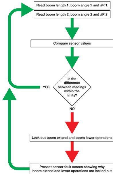
Redundant sensor process
