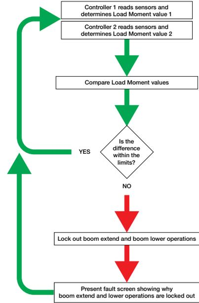
Redundant controller process
