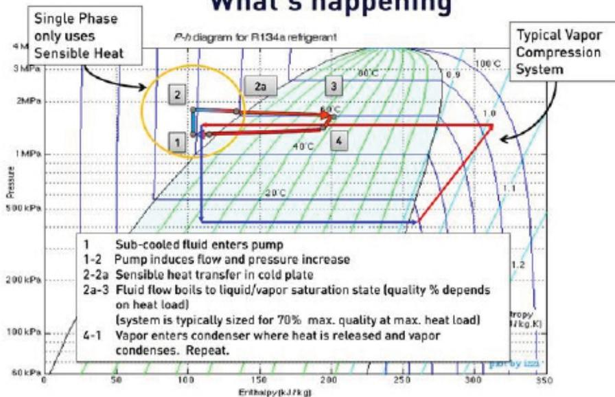
The enthalpy chart illustrates how the system works and how we achieve our performance gains. The lines are exaggerated for clarity and here we are comparing our pumped 2-phase system against a classic vapor compression system. In our system the fluid enters the pump at point #1, there is a small pressure rise and from point 2-2a the fluid picks up sensible heat. This triangle, 1-2-2a-1 is the only region single phase water loops operate in.
