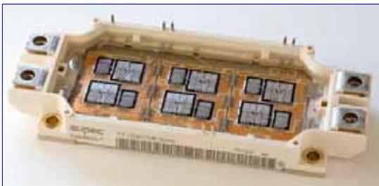
**Figure 2:** IGBT power semiconductor module (1200V 450A)
