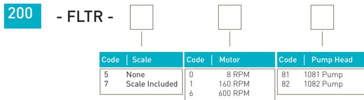
Example: 200-FLTR-7181 - SciLog® FilterTec™ - with scale, 160 RPM motor and 1081 head
