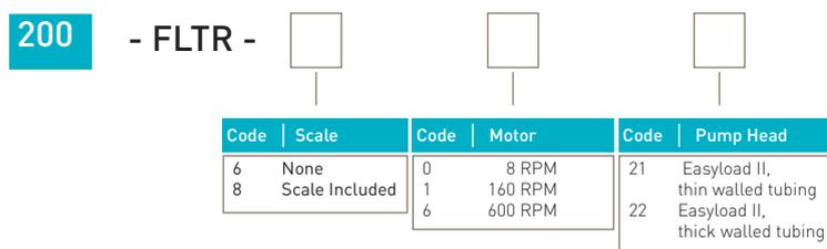
Example: 200-FLTR-8121 - SciLog® FilterTec™ Plus - with scale, 160 RPM motor and 3 MasterFlex Easyload II heads for thin walled tubing.
