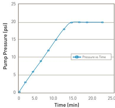
**Fig. 2 - FilterTec™ R/P Programmable Mode Time-Programmable Pump Pressure**
