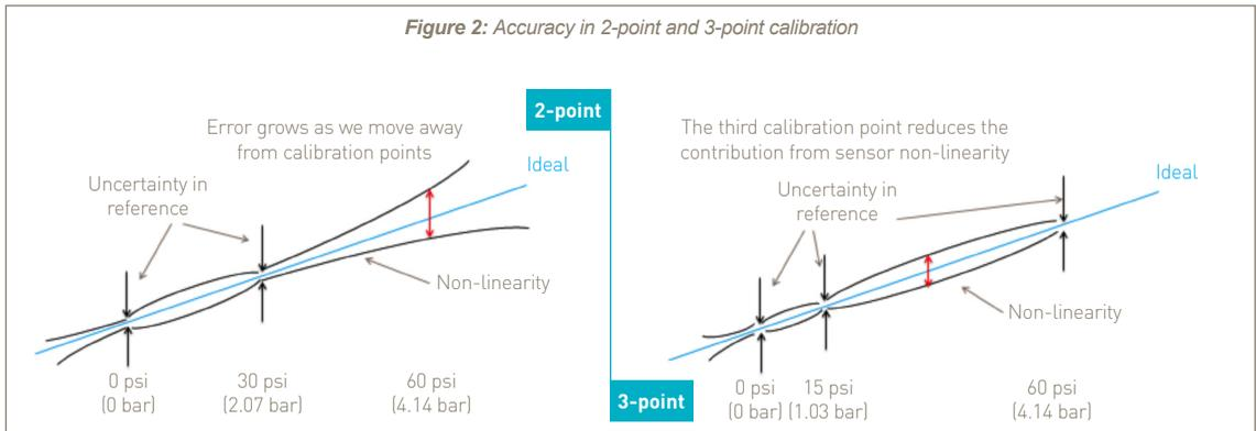
the actual pressure value. A single sensor with a fixed systematic error (or bias) will report true changes in pressure if the error doesn't change. While specific claims about the precision of sensors are not made, data indicates precision is even better than accuracy.
