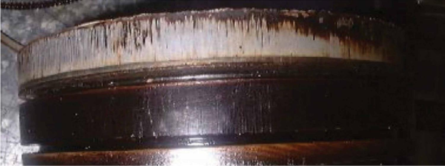
Fig 4 – Contamination of engine oil
