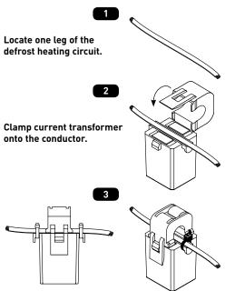
Apply 0.1" wide zip-ties to secure Current Transformer to line.
