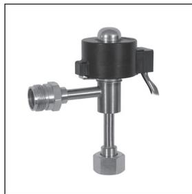
The Parker SEV-C is a unipolar EEV with internal check feature for use in reverse flow applications, (i.e. residential heat pump systems). The check valve allows flow to bypass the expansion port in reverse flow when the valve is fully open. This minimizes liquid pressure drop. SEV-C features include:
