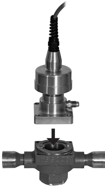
4. Install the new bolts supplied with the adaptor. Tighten in a star cross pattern to 10-foot pounds of torque.
