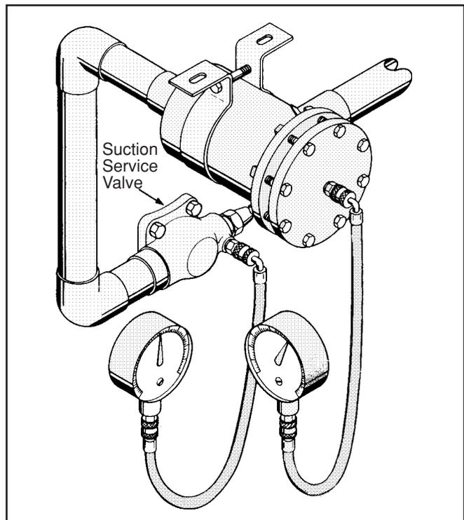
The filter elements (purchased separately) are installed in place of the cardboard spacers shipped with the unit. Detailed instructions for installing the elements are given on the filter element package. Inspect the edge of the shell and the gasket surface immediately before installing the flange plate to obtain a clean, leak-tight joint. A new gasket is supplied with each filter element. It is recommended that this gasket only be replaced if it is damaged.
