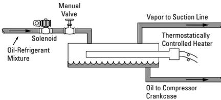
**ELECTRIC HEATER** - may also be used to separate oil and refrigerant. This system is similar to that of Figure 6 except that heat required for vaporization is added electrically.
