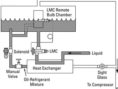
**OIL RETURN** - by draining oil-refrigerant mixture through a heat exchanger is illustrated here. Heat in incoming liquid vaporizes refrigerant to prevent return of liquid to compressor. Liquid feed is controlled by a hand expansion valve.
