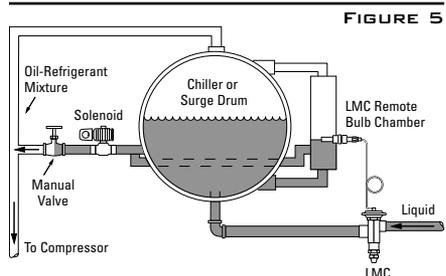
**DIRECT DRAIN** - of oil to the suction line is one of three ways to recover oil in flooded systems. Heat from the environment or a liquid-suction heat exchanger is required to vaporize the liquid refrigerant so drained. Vapor velocity carries oil back to the compressor.
