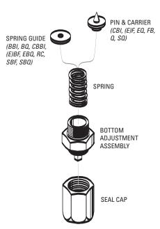
**KA-1** for Valve Type A **KA-6** for Valve Types K,
