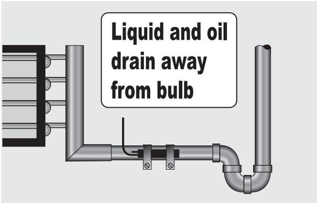
The sensing bulb should be securely fastened to a clean, horizontal section of the suction line at the evaporator outlet.
