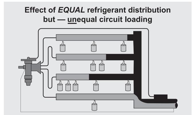
*These illustrations depict conditions that result in a loss of heat transfer due to either (top) unequal circuit loading or (bottom) unequal refrigerant distribution.*
