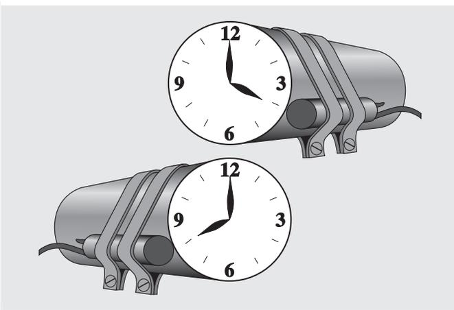
On suction lines 7/8" and larger, the sensing bulb should be installed at 4 or 8 o'clock on the side of the horizontal line.
