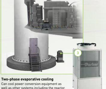
transformer, and generator. Enables up to twice the power density or up to 40% higher throughput from existing electronics at a lower system cost.
