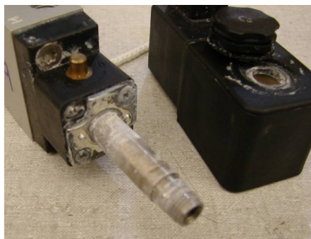
Figure 8: Salt Spray Testing performed on pilot operator and coil
