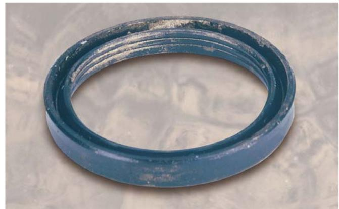
**SYMPTOMS:** Rod seals and bearings are worn on one side only (Fig. 1). Piston rods and cylinder tubes are worn or galled on opposite sides, particularly at or near full extension (Fig. 2). Piston rods should be straight within 0.15mm per metre; T.I.R. and surface finishes should be below 0.4 microns R.M.A.
