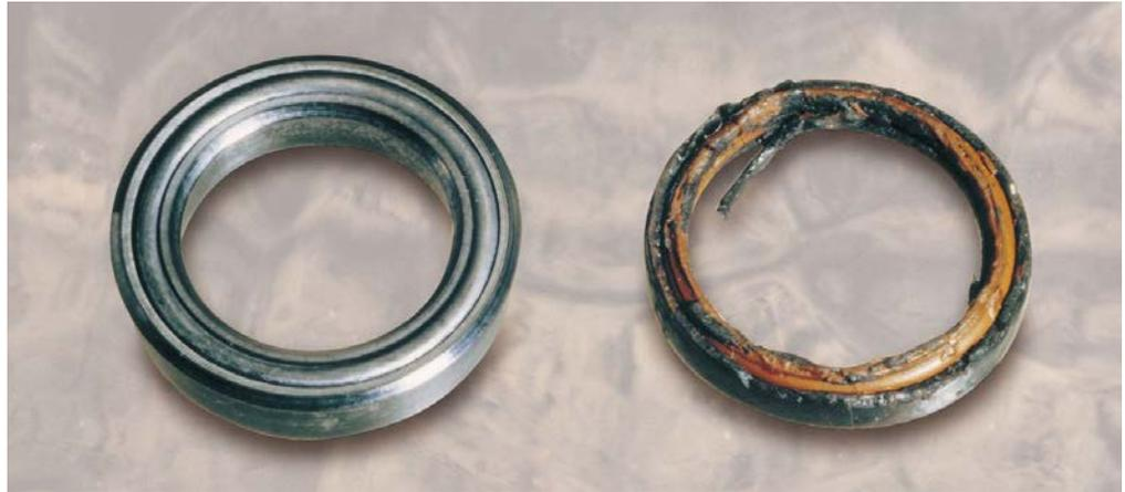
**SYMPTOMS:** Seals feel sticky or gummy in some cases, or may appear dry and cracked (Fig. 7). Shrunken seals may rattle in their cartridge grooves, while swollen seals may prove difficult to remove from the cylinder.
