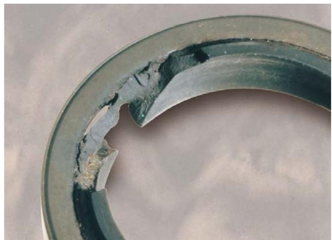
**SOLUTION:** If excessive pressure is caused by intensification due to a flow restriction, the restriction should be removed. If the condition persists, a special gland and seal design should be
