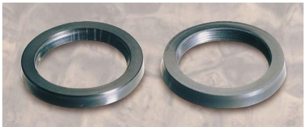
**Fig.3 Contamination damage is apparent in this rod seal, where the serrations are worn completely away. The seal on the right is a new one, shown for comparison.**
