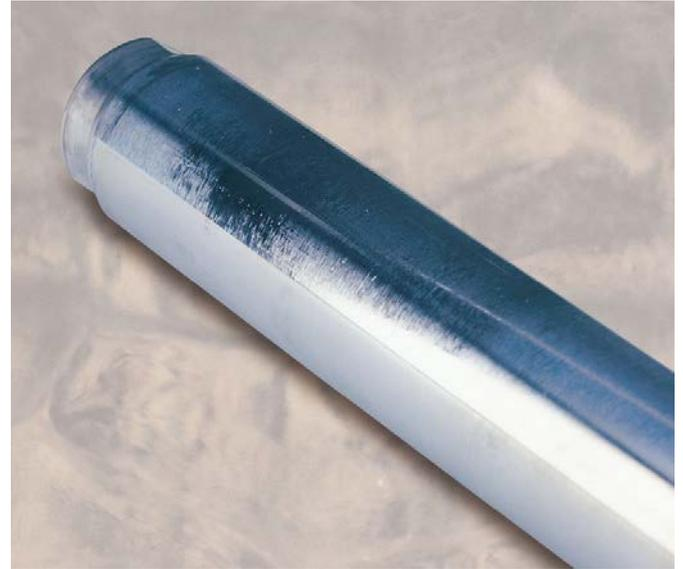
**Fig.2 Galling on this piston rod is evidence of excessive side loading.**
