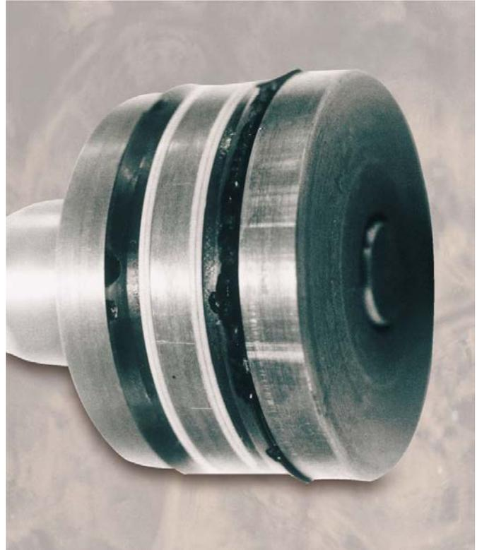
**Fig.5 Piston seals damaged by air in oil.**
