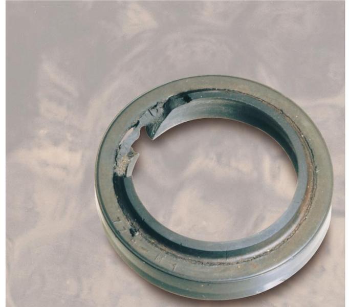
**Fig.9** The rod wiper may extrude (top) but the primary rod seal looks perfect (right), so no leakage occurs when the cylinder is hydrostatically tested.
