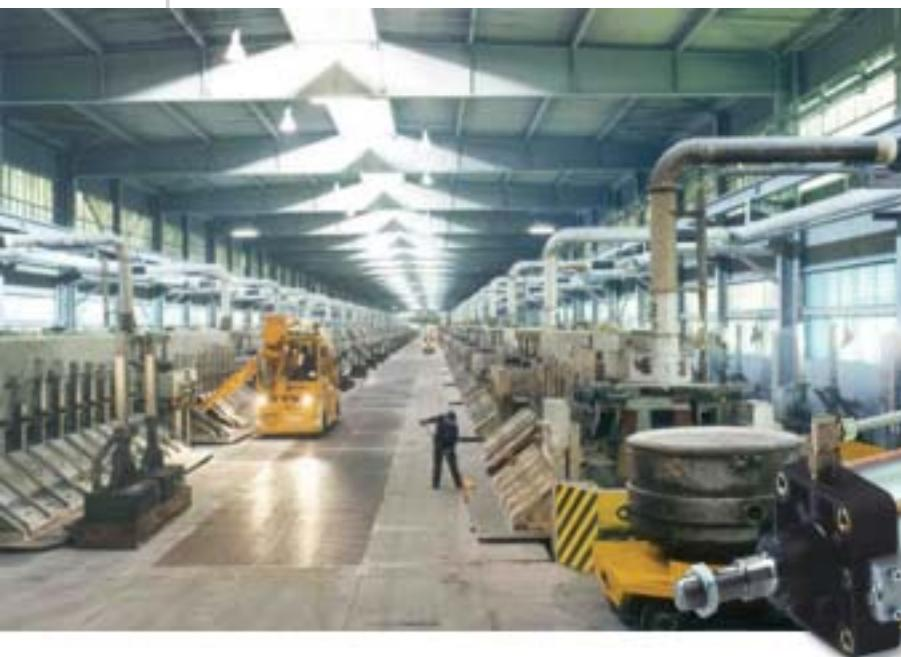
Our Intelligent Crustbreaker cylinder saves up to 70% in compressed air based on proven technology from the C40 series. A complete working unit determines:
