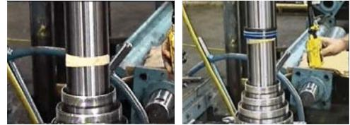
Or extend the plunger or sleeve out about one foot. Wrap masking tape around a clean area on the plunger or sleeve. Push plunger or sleeve back into and past the packing and pull out. Packing will usually pop out, if not, repeat the process.
