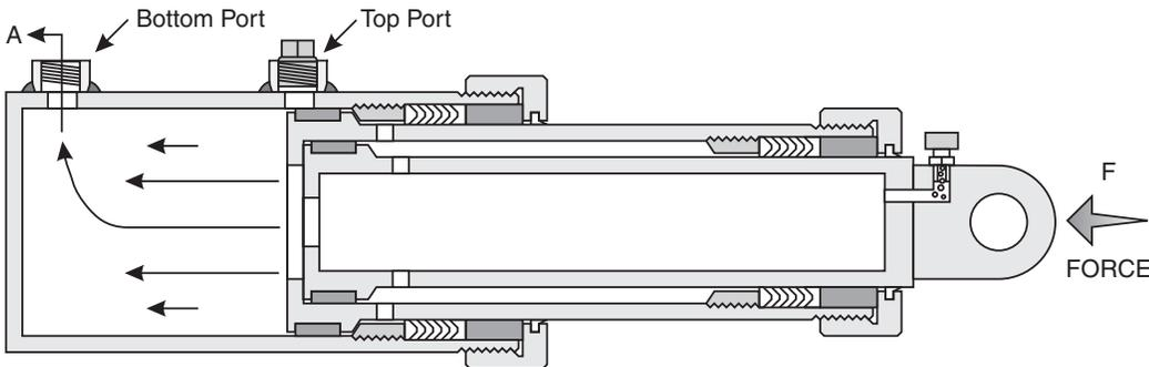
**Note:** If the top port is used, the speed of the cylinder may be reduced because of the oil flow restriction as the oil passes thru the transfer holes (G).
