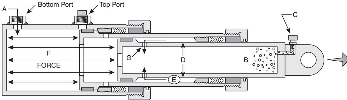
So at a given PSI (pressure) and GPM (gallons per min.) the cylinder will develop less force and increase in speed as it changes to the next moving stage.
