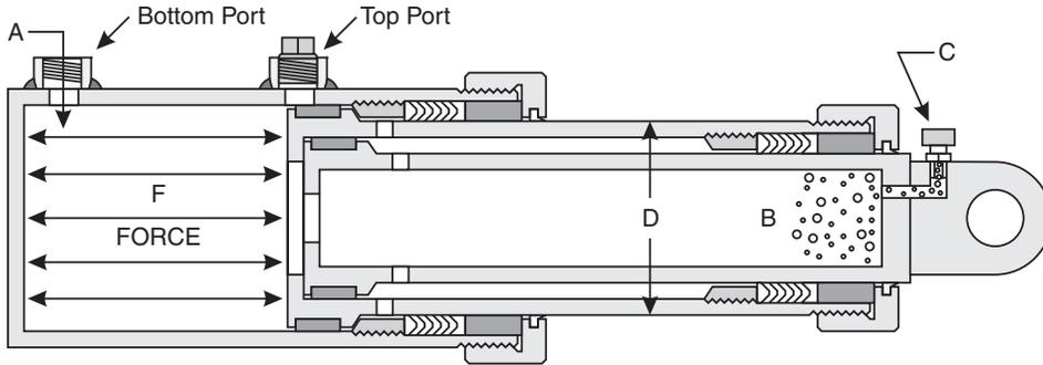
As the sleeve or plunger moves out, the oil trapped between (E) the sleeve or plunger wall is released through transfer holes (G) which are drilled in the sleeve or plunger.
