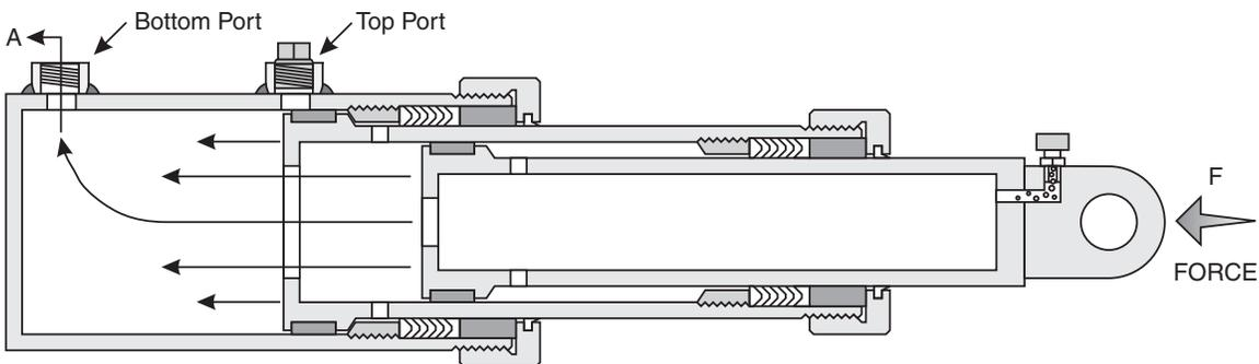
Under normal operating conditions the plunger or smallest diameter sleeve is pushed closed first, forcing oil out through port (A), then the next smallest, etc.
