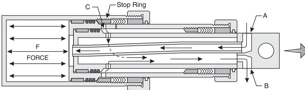
The effective area of each stage is figured from the inside diameter of the next largest stage. Each stage extends in its turn to the stop ring. So at a given PSI (pressure) and GPM (gallons per min.) the cylinder will develop less force and increase in speed as it changes to the next moving stage.
