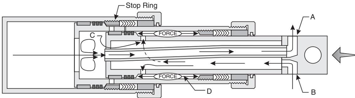
retracts in its turn, however, THE EFFECTIVE AREA FOR RETRACTING EACH STAGE IS THE AREA (D) OF THE PLUNGER.
