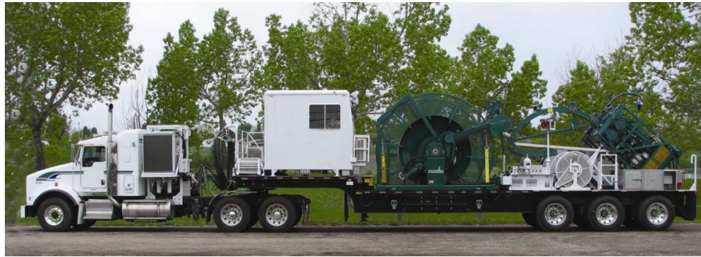
Coiled Tubing Unit
