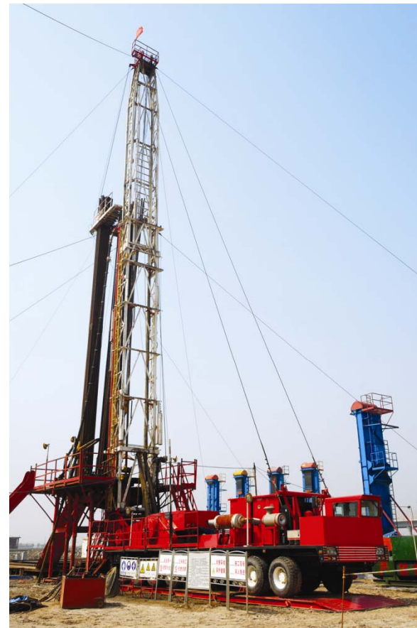
Well Service Rig
