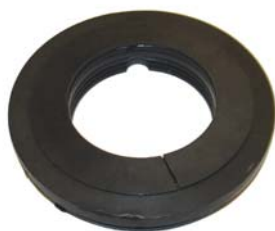
Failed Seal Resulting from Improper Fit
