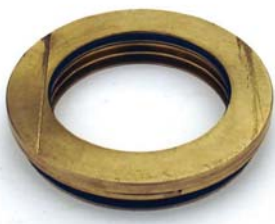
Failed Seal Resulting from Improper Installation
