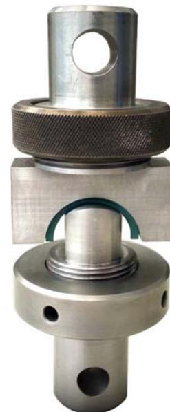
Figure. 2: Custom fixture for testing wear ring compressive modulus
