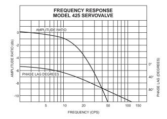
Valve rated at 25 GPM @ 1000 psi drop. Supply pressure 3000 psi
